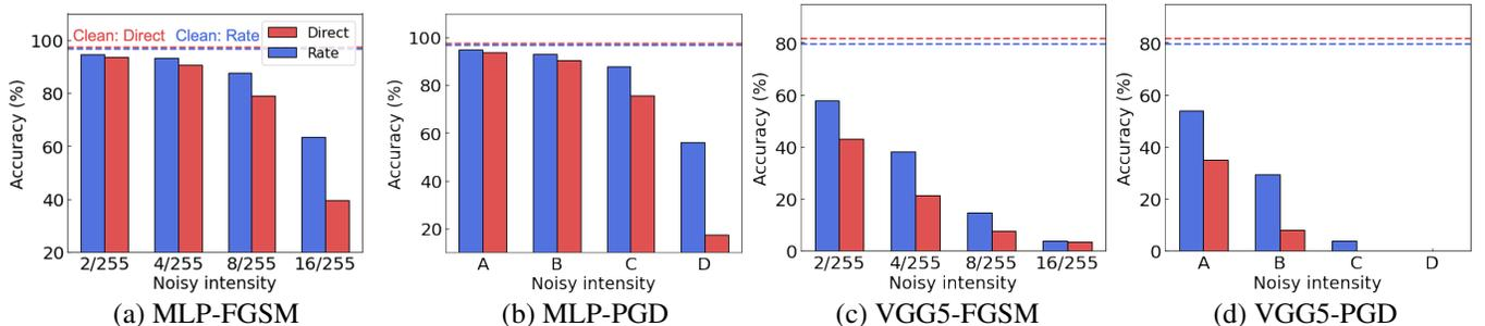
**Fig. 3.** The adversarial robustness with respect to FGSM attack and PGD attack. We present the clean accuracy using dotted lines. In the PGD attack experiments, A-PGD[2/255, 1/255,10], B-PGD[4/255, 1/255,10], C-PGD[8/255, 4/255,10], D-PGD[16/255, 4/255,10]. We use timestep 10 for all experiments.
