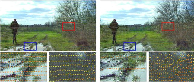
**Fig. 2.** The visual comparison of point clouds from high-resolution LiDAR and low-resolution LiDAR. The point cloud is projected to the image plane and plotted as an overlay layer. The data is from RELLIS-3D[17]. **Left:** 64-channel LiDAR. **Right:** 32-channel LiDAR. **Blue box:** sparse region. **Red box:** noisy region.
