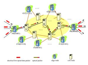
Fig. 1. An optical core network with 32 edge nodes.
