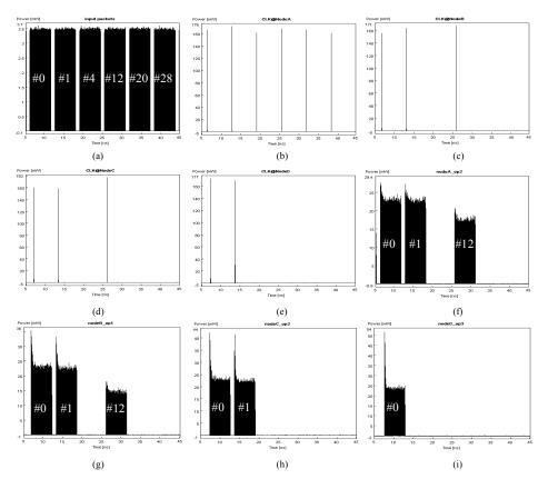
Fig. 6. Time waveforms; (a) input packet at node A, (b)-(e) extracted clock at nodes A, B, C, and D, and (f)-(i) switched packets at nodes A – output2, B – output1, C – output2, and D – output3.
