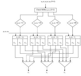
Fig. 2. A block diagram of multiple PPRT ( $E_{1A}$ ,  $E_{2A}$ ,  $E_{3A}$ , ...,  $E_{3D}$ ) for 5-bit packet header address.
