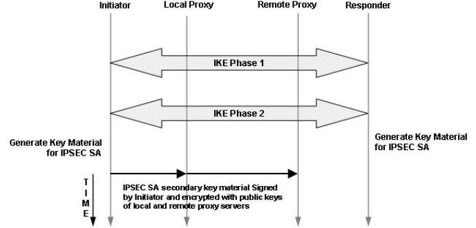
Fig. 2. Addition to IKE handshake mechanism for LES key management
