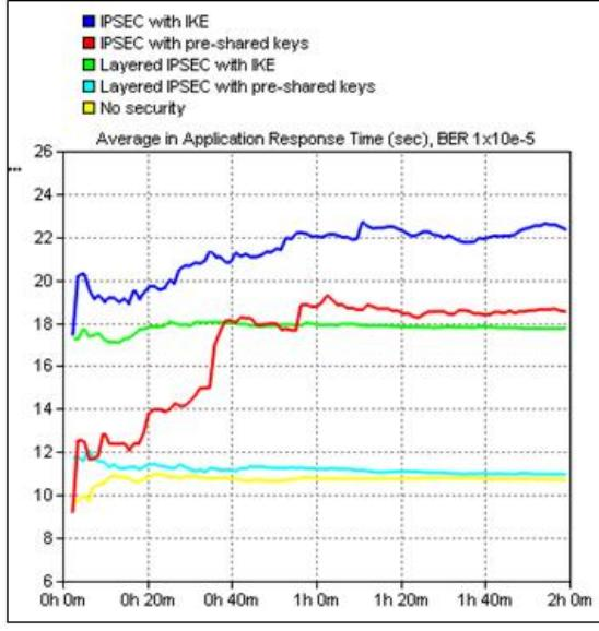
Fig. 4. Comparison of custom application response time (global average) for satellite link  $\text{BER } 1 \times 10^{-5}$ .
