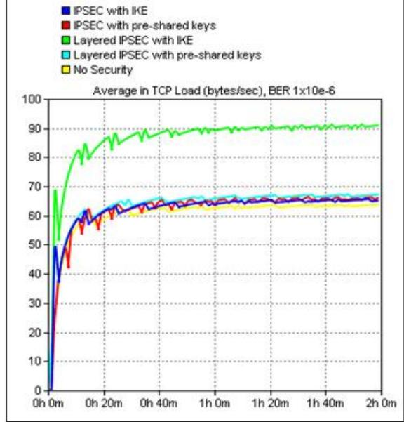
Fig. 5. Average TCP load at client for  $\text{BER } 1 \times 10^{-6}$ .
