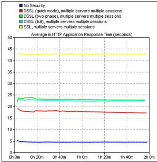
Fig. 8. HTTP response times for different versions of DSSL and comparison to SSL and unsecured web browsing.
