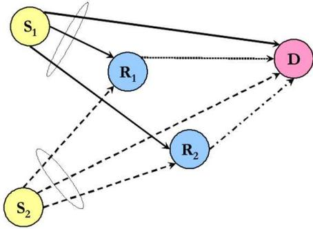
Fig. 1. Two-source two-relay network topology. Different line-styles denote transmission over orthogonal channels (e.g., time-slots) to avoid mutual interference:  $S_1$  transmits in time-slot 1 (solid lines),  $S_2$  in time-slot 2 (dashed lines),  $R_1$  in time-slot 3 (dotted lines), and  $R_2$  in time-slot 4 (dashed-dotted lines).
