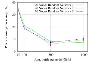
Fig. 1. Power consumption savings versus traffic for different sized networks.
