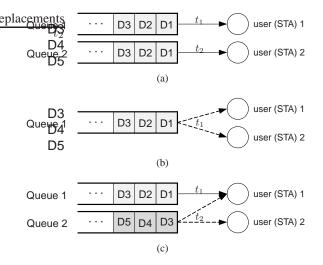
Fig. 1. Illustration of (a) unicast. (b) multicast. (c) opportunistic multicast.
