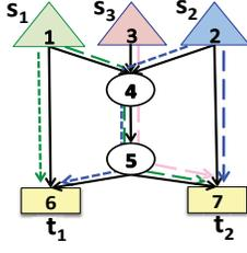
Fig. 2: Illustration of a feasible solution to Problem 1.  $\mathcal{P} = \{1, 2, 3\}$ ,  $\mathcal{S} = \{s_1, s_2, s_3\}$ ,  $R_1 = R_2 = R_3 = 1$ ,  $B_{ij} = 2$  for all  $(i, j) \in \mathcal{E}$ ,  $\mathcal{T} = \{t_1, t_2\}$ ,  $\mathcal{P}_1 = \{1, 2\}$  and  $\mathcal{P}_2 = \{1, 2, 3\}$ . Thus,  $\mathcal{Y} = \{\{1, 2\}, \{3\}\}$ ,  $L_{\max} = |\mathcal{Y}| = 2$  and  $L \in \{1, 2\}$ .
