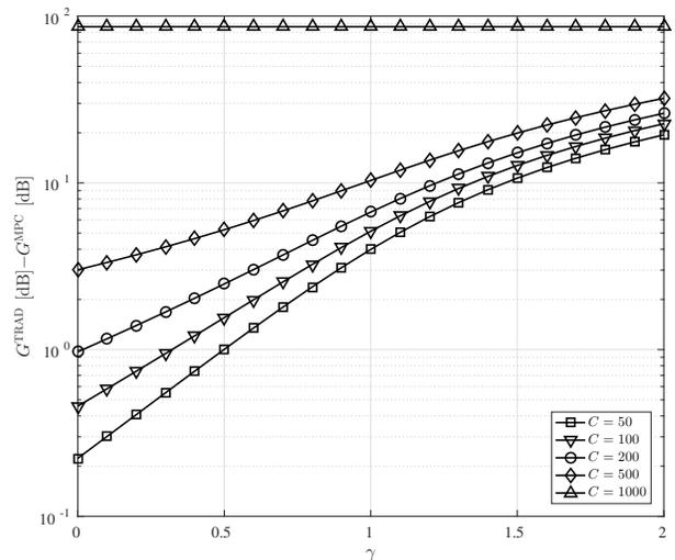
Fig. 3. Coding gain gap between the traditional and MPC schemes;  $K = 6$ ,  $R_F = 2.5$  bps/Hz.
