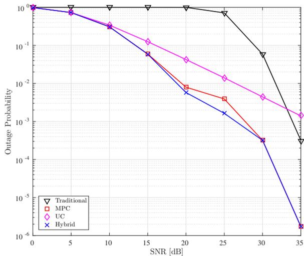
Fig. 2. Comparison of outage probability with different schemes;  $K = 6$ ,  $\gamma = 2$ ,  $R_F = 2.5$  bps/Hz; solid lines depict the theoretical results.
