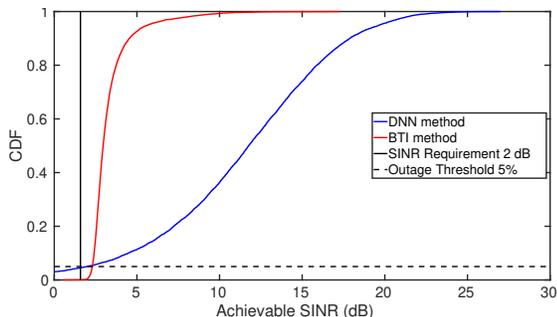
Fig. 2. The CDF performance comparison between the BTI method and the proposed DNN method for user 1 in a  $2 \times 2$  scenario.
