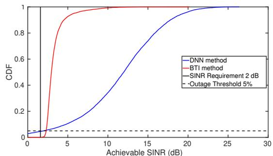
Fig. 3. The CDF performance comparison between the BTI method and the proposed DNN method for user 2 in a  $2 \times 2$  scenario.
