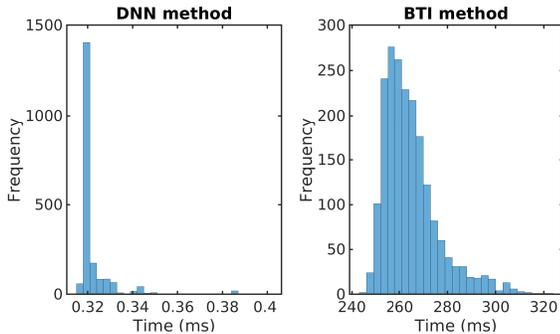
Fig. 4. The frequency of the 2000 execution time performance, compared between the proposed DNN method and the BTI method.
