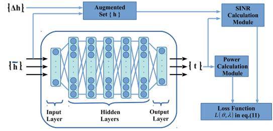
Fig. 1. An illustration of the proposed DNN training method for the robust beamforming problem in the URLLC networks.
