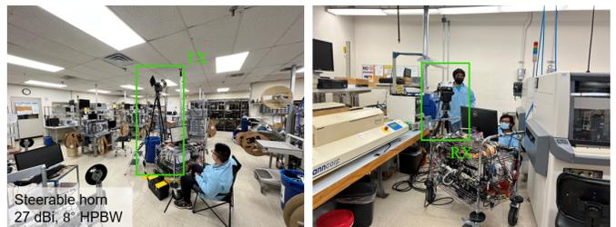
Fig. 2: Photos taken from Factory B. The TX was set at 2.5 m, and the RX was set at 1.5 m.
