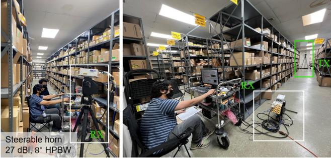
Fig. 3: Photos taken from Factory C. The TX was set at 2.5 m, and the RX was set at 1.5 m and 0.5 m.
