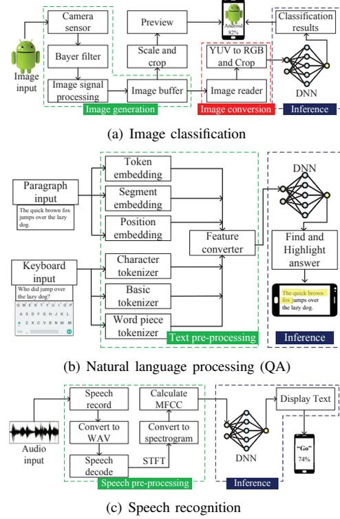
Fig. 2. Pipelines of the mobile AI applications studied in this research. and position embeddings. The keyboard input goes through character, basic, and word piece tokenizer. These embeddings and tokens are passed to a feature converter providing input to the DNN model. The model finds the answer to the question input and highlights it in the paragraph.
