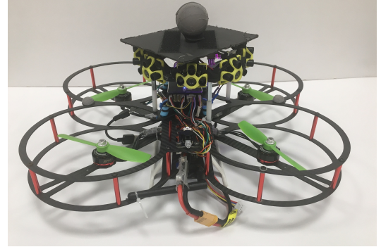
Fig. 10. UAV Mechanical Overview.
