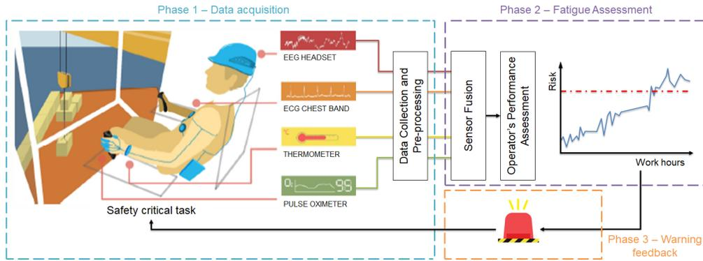
Fig. 1. Proposed sensor framework for fatigue assessment.
