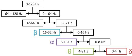
Fig. 2. DWT filter bank.
