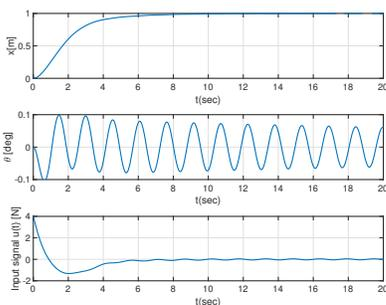
Fig. 5. Energy-based control: position  $x$ , payload swing  $\theta$ , and control  $u(t)$
