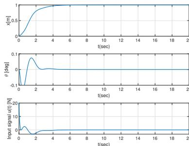
Fig. 7. ASMC: position  $x$ , payload swing  $\theta$ , and control  $u(t)$
