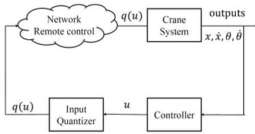
Fig. 3. Crane control with input quantization over a network
