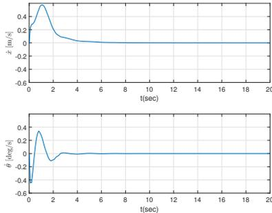
Fig. 10. Quantized ASMC: velocity  $\dot{x}$ , payload swing speed  $\dot{\theta}$
