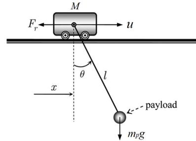
Fig. 2. Illustration of an underactuated crane [13]
