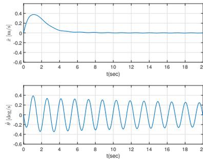
Fig. 6. Energy-based control: velocity  $\dot{x}$ , payload swing speed  $\dot{\theta}$
