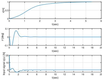
Fig. 9. Quantized ASMC: position  $x$ , payload swing  $\theta$ , and control  $u(t)$
