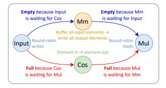
Fig. 5: An example of a computation graph that causes deadlock with default FIFO sizing for any non-trivial input. The root cause is the contention between the "Mm" which buffers elements with a delay before writing out data and "Cos" which writes out data every cycle.
