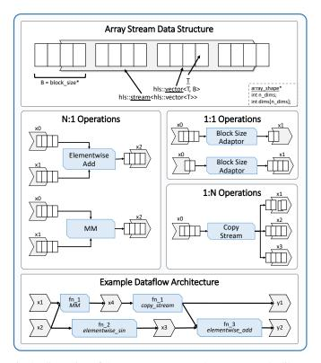
Fig. 3: Illustration of the array\_stream data structure, the library of stream-based kernels, and an example compute graph mapped to a dataflow architecture.
