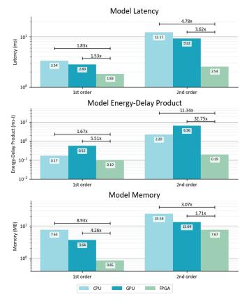
Fig. 7: Main comparison results for latency, energy-delay product, and memory of 1st-order and 2nd-order INR models between GPU, CPU, and the proposed FPGA implementation. The y-axes are log scales.
