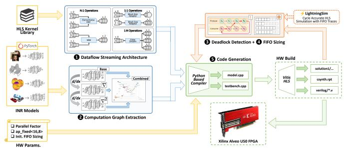
Fig. 2: An overview of the INR-Arch framework for end-to-end hardware acceleration for INR editing based on the INSP-Net [12] architecture.
