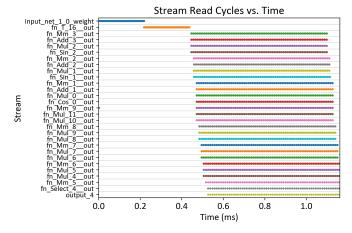
Fig. 8: A trace of FIFO reads for a representative subset of hardware computation kernels in the main dataflow region of the Base INR + 1<sup>st</sup> Order Gradient INR-DSP model.
