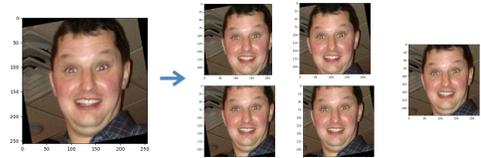
Fig. 6. Image Rescaling to 256x256 pixels initially. Five images are extracted from each four corners and centre which are resized to 224x224 for feeding into the network.
