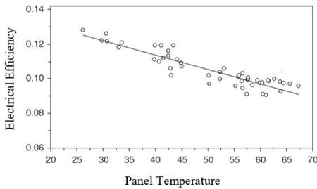
Fig. 3. Relation between electrical efficiency and panel temperature
