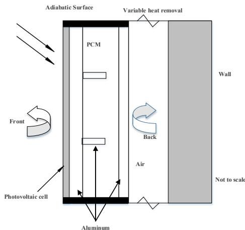
Fig. 6. PV Panel with PCM [11]
