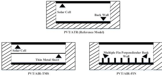
Fig. 2. Different cross sectional view of PVT/AIR model
