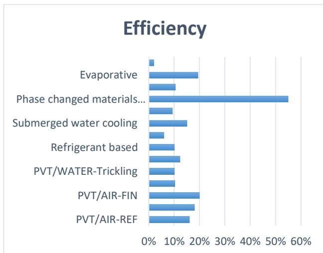
Fig. 7. Comparison of efficiency for different cooling technique
