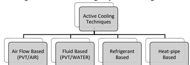
Fig. 1. Different cooling techniques
