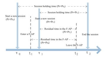
Fig. 3. Timing Diagram For Mobility Model.
