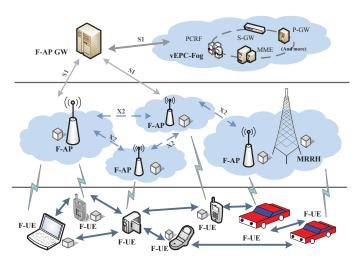
Fig. 1. A NFV-based FRAN Architecture.
