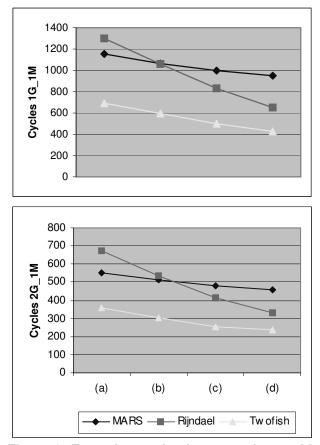
Figure 3. Execution cycles in one and two-wide processors with one memory port. (a) Indexed (b) Scaled-indexed (c) Scaled-indexed + extract (d) load.ex.sc.
