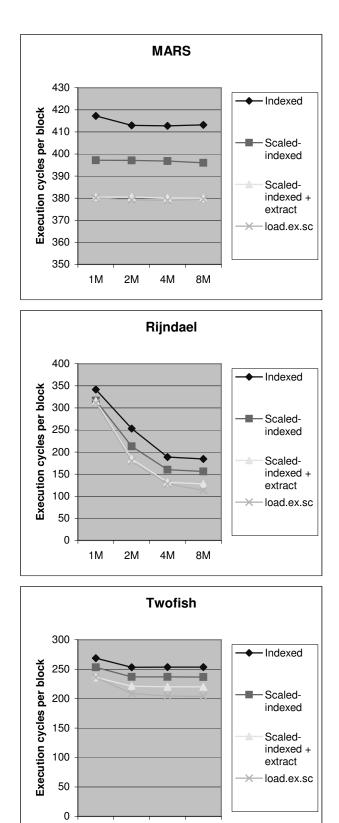
Figure 4. Execution cycles for one, two, four and eight memory ports in an eight-wide processor.
