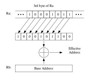
Figure 2. load. 3b.4 Rd, Ra (Rb)
