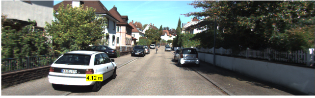
Figure 5. Distance estimation based on the computed depth. First top image represents the original RGB image from a video sequence. The image at the middle shows the estimated depth map using the proposed method. The last image shows an object labelled with its distance to the camera based the depth map.
