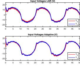
Fig. 10. Voltage for test 3 with disturbance of changing tail propeller
