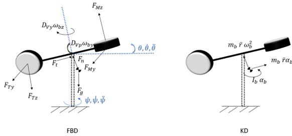
Fig. 2. Free body diagram and kinetic diagram of the Aero body
