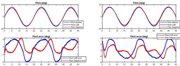
Fig. 5. Pitch angle and error for test 2 with disturbance. Left: negative torque; right: positive torque
