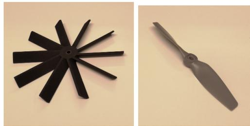
Fig. 8. Propellers: Left-low efficiency, Right-high efficiency
