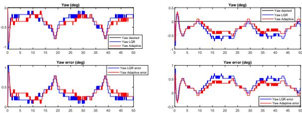
Fig. 6. Yaw angle and error for test 2 with disturbance. Left: negative torque; right: positive torque
