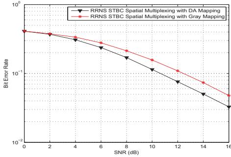
Fig. 7. Comparison of BER performance of Spatially Multiplexed RRNS(6,3)- STBC ( $T = 3$ ) with prior probability based Distance-Aware mapping and Gray coded mapping assuming equal priors
