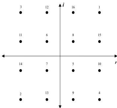
Fig. 4. Probability Based Distance-Aware Mapping Scheme for 16-QAM
