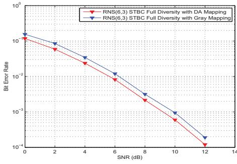
Fig. 6. Comparison of BER performance of Full Diversity RRNS(6,3)-STBC ( $T = 3$ ), with prior probability based Distance-Aware mapping and Gray coded mapping with ML decoding assuming equal priors
