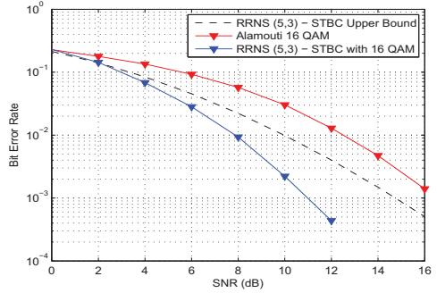
Fig. 5. BER performance of RRNS (5,3)-STBC with moduli set of  $m_o = \{7, 9, 11\}$ ,  $m_r = \{13, 16\}$ .
