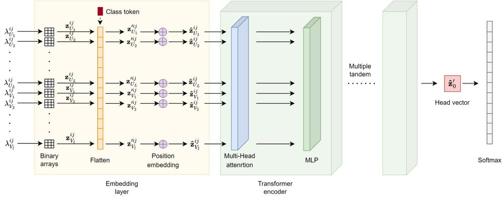
Fig. 4. The diagram of ViT based model selector
