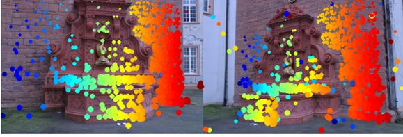
Figure 3. Putative matches obtained with the classical SIFT algorithm, which seeks matches over the entire image. The figure shows images 7 and 3 from the Fountain dataset.
