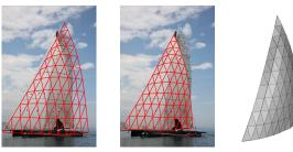
Figure 15. Image registration and surface reconstruction on the sparsely textured sail surface. From left to right: input image and initialization; final registration and reconstruction; the sail shape seen from a different viewpoint.
