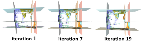
Figure 5. Joint optimization procedure. As we iterate layout estimation and global registration procedures, the fragmented structures merge into a wall region.
