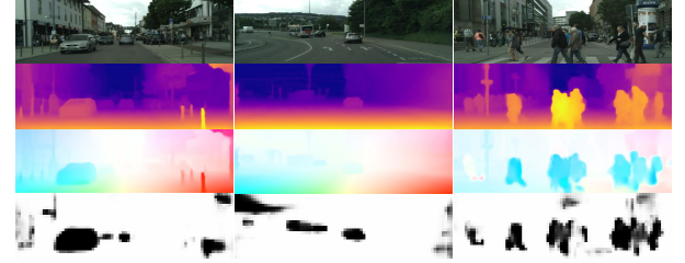
Figure 8: Generalization test on Cityscapes [8]. From top to bottom: input first frame, estimated depth of first frame, synthesized optical flow, estimated rigidity soft mask.
