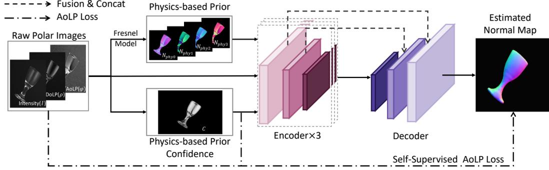
Figure 2. **Overview of our proposed method.** We use a multi-branch architecture to handle different hierarchical inputs rather than directly concatenating them. The physics-based prior confidence map is defined from raw polarization images and used for the weighted fusion of different inputs. In addition, we propose the self-supervised AoLP loss by exploiting the confidence map to force the network to learn the prior knowledge between the normal and AoLP
