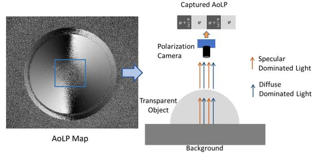
Figure 4. **The characteristic in the AoLP map of the transparent surface.** The noise in the AoLP map is derived from the transition between specular dominance and diffuse dominance on the background surface. More noise indicates higher transmittance and also lower reliability of physics-based prior
