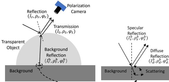
Figure 3. **Different components captured by polarization camera.** The captured ray consists of reflection and transmission components, where the transmission component is composed of two kinds of reflections from the rough background
