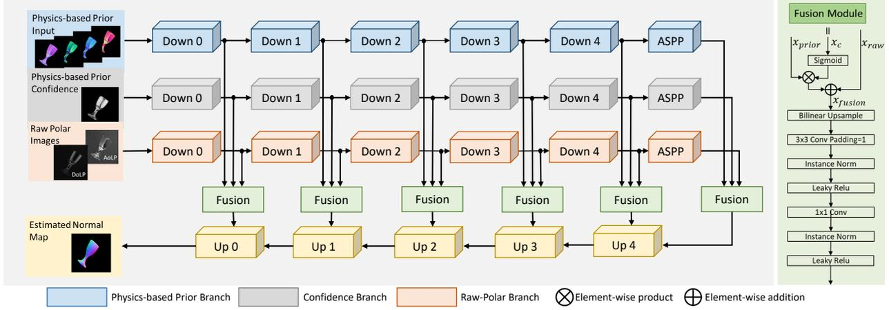
Figure 5. **Overview of TransSfP.** We regard raw polar images, physics-based prior, and confidence map as different hierarchical information and input them into three independent encoders. The confidence branch is used for weighting the features from physics-based prior branch, which is completed in our proposed fusion module
