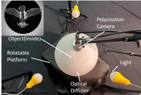
Figure 6. Setup for acquiring real-world dataset
