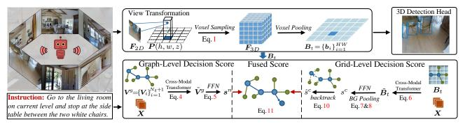
Figure 2: Overview of BSG. View transformation is first employed to project the multi-view images into BEV plane (§3.1). Then, BEV feature is encoded using 3D detection (§3.3). Through the integration of BEV representations during navigation, we predict a graph-level decision score on BSG and a grid-level decision score based on BEV. These scores are fused to facilitate effective decision-making (§3.2).
