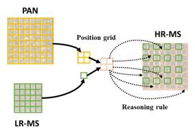
Figure 1: **Motivation.** Pan-sharpening is to reason the unknown content at the pre-defined pixel positions according to the context of low-resolution multi-spectral image and high-resolution panchromatic image.
