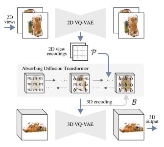
Figure 1. The proposed approach independently learns a discrete information-rich codebook for 2D and 3D domains with two VQ-VAEs. New 3D samples are then synthesized conditional on the complete codebook of multiple 2D views with a transformer.
