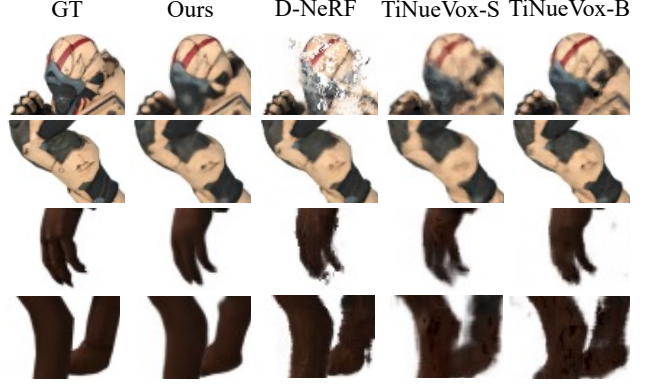
Figure 5. Qualitative comparison on D-NeRF Dataset. We show some novel view synthesized images on the selected test set of the dataset. Comparing ours with ground truth, D-NeRF [36] and TiNeuVox [10]. Our model yields cleaner images with more details.
