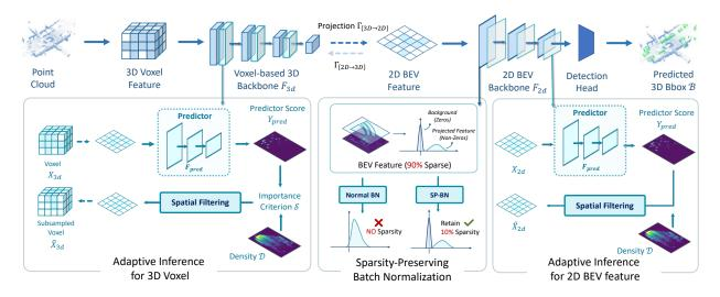
Figure 3: **The overall framework of Ada3D.** Adaptive inference is conducted in both the 3D and 2D backbone. The spatial filtering module combines the predictor score and 3D point cloud's density to drop the redundant parts. Furthermore, the SP-BN is introduced to omit the background pixels in 2D backbone and retain sparsity.
