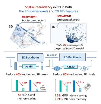
Figure 1: Ada3D is an adaptive inference framework that exploits the spatial redundancy for both the 3D voxel and 2D BEV features.
