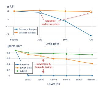
Figure 2: **Empirical evidence of spatial redundancy in 3D and 2D data.** Upper: The KITTI Cars Moderate AP under different drop rates with random dropping and ground-truth excluded dropping. Lower: The sparsity of different layer's 2D BEV features.
