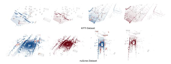
Figure 11: Visualization of the 3D point cloud colored by predicted importance score for different datasets. The orange represents higher importance, and the blue stands for the lower. The red points stand for dropped points given a high drop rate.
