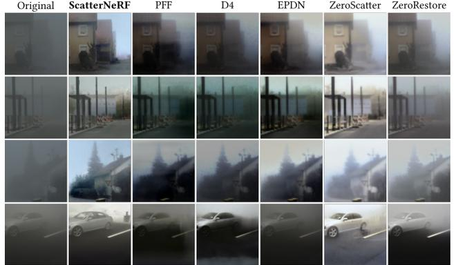
Figure 5: Qualitative comparison of dehazed images on real-world automotive measurements. The proposed ScatterNeRF enables enhanced contrast and visibility compared to state-of-the-art descattering methods.
