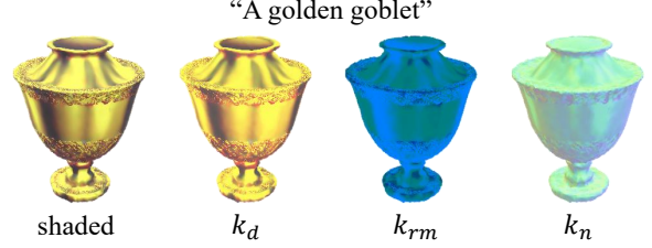
Figure 4. Three components of the material model, namely the diffuse term k_d , the roughness and metallic term k_{rm} , and the normal variation term k_n .
