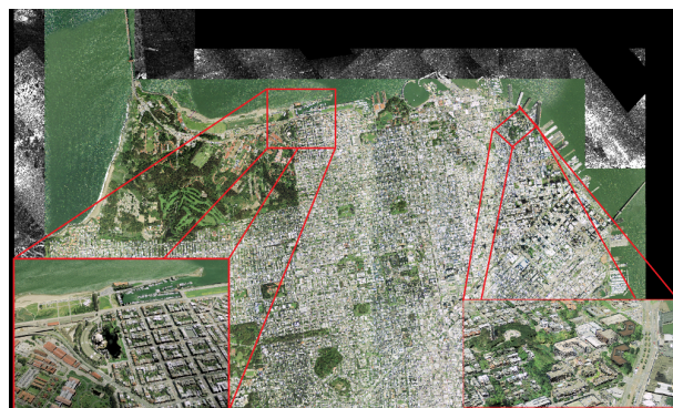
Figure 1. Point based rendering of a large scale LiDAR dataset textured with high resolution ortho-imagery. LiDAR datasets served as our reference model for the exact geo-referentiation of camera images from community video and image collections.
