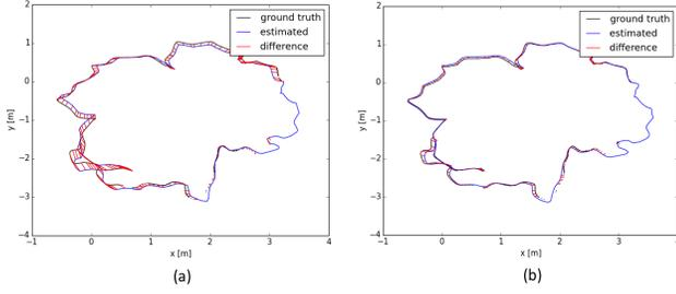
Figure 8. Estimated camera trajectory comparison on *fr2\_xyz* [32] sequence. (a) Before loop closing. The RMS of ATE is 9.5 cm. (b) After loop closing. The RMS of ATE is 1.75 cm
