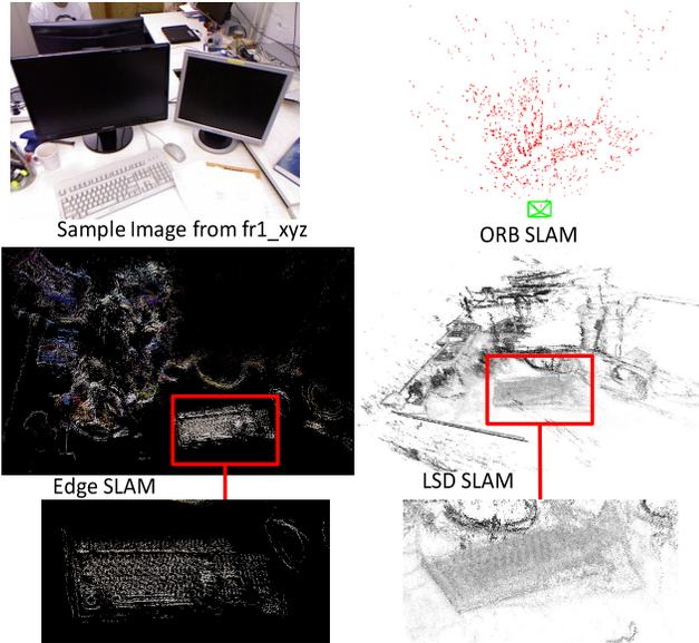
Figure 9. The figure shows comparisons among reconstructed structures by ORB SLAM, LSD SLAM and our Edge SLAM on *fr1\_xyz* [32] sequence. ORB SLAM structure is too sparse to understand the environment. LSD SLAM generates a semi-dense structure, where multiple overlapped structures are visible. Our Edge SLAM generates a 3D structure which yield semantic understanding of the environment.
