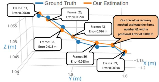
Figure 7. Validation of track-loss avoidance in *fr3\_str\_notex\_far* [32] sequence. Camera estimation become unreliable as 3D-2D correspondences become very low at frame number 61. Our track-loss recovery method estimates the frame with 0.3 cm absolute positional error against ground-truth.
