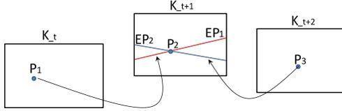
Figure 3. Three view validation of correspondence.  $EP_1$  and  $EP_2$  are the corresponding epilines [10] for points  $P_1$  &  $P_3$  respectively. If point  $P_2$  holds feature correspondence with  $P_1$  &  $P_3$ , it should be the intersection point of  $EP_1$  &  $EP_2$ .
