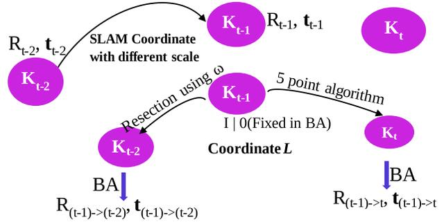
Figure 6. Track-loss recovery: Images  $K_{t-2}$ ,  $K_{t-1}$  and  $K_t$  are estimated separately in  $L$  coordinate and these estimations are transformed to SLAM coordinate by coordinate merging after scale correction.
