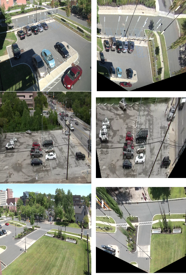
Figure 8: (Left) Source images (Right) Bird’s eye view of the corresponding source images which are automatically calculated using our method.
