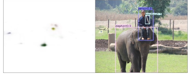
Figure 3: Raw heatmaps from anchor-free detection prediction (left) and their corresponding predicted boxes (right) after box offset, size and thresholding.
