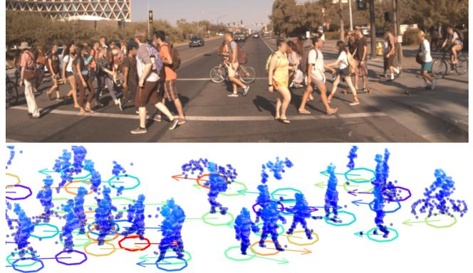
Fig. 1. Association and tracking of pedestrians is challenging in dense, urban environments. We propose a real-time learned association and tracking system with IMM filtering that incorporates LiDAR + camera modalities that improves both on the task of association and state estimation.
