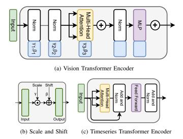
Fig. 4: Architecture of the encoder blocks and Scale and Shift block.
