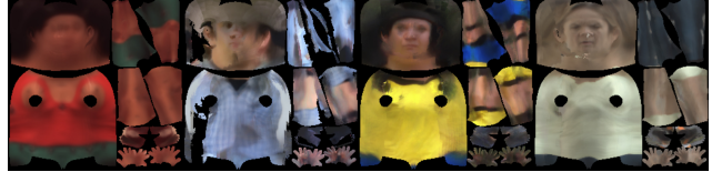
Figure 3. Examples of reconstructed texture maps from Human3.6M, 3DPW and RICH used for training and evaluation. We generate texture maps by back-projecting the image colors from multiple frames to all visible vertices.
