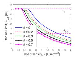
Fig. 3: Limit on Zone 0 radius based on the handover requirements as a function of the user density,  $\epsilon$ , for different values of  $\beta$  when  $\theta_1 = 60^\circ$ ,  $B_{\text{HO}} = 10$  Kbits, and  $N_{\text{cell}} = 64$ .
