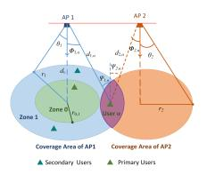
Fig. 1: General system model of a cognitive VLC scenario, comprised of two LED-based access points (*i.e.*, AP1 and AP2) and multiple mobile users.
