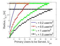
Fig. 4: Minimum (solid lines) and maximum (dashed lines) values of radius of Zone 0 that can satisfy both handover and illumination requirements as a function of the primary users to be served for different values of  $\epsilon$ , when  $\theta_1 = 60^\circ$ ,  $B_{\text{HO}} = 10$  Kbits, and  $\beta = 0.4$ . Herein,  $\Lambda_{0,1} = 3.5$  m and  $\lambda_{0,1} \approx 3$  m.
