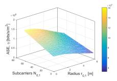
Fig. 2: Area spectral efficiency of AP1 as a function of both  $r_{0,1}$  and  $N_{0,1}$  when  $\theta_1 = 60^\circ$  ( $r_1 \approx 6$  m) and  $N_{\text{cell}} = 64$ .
