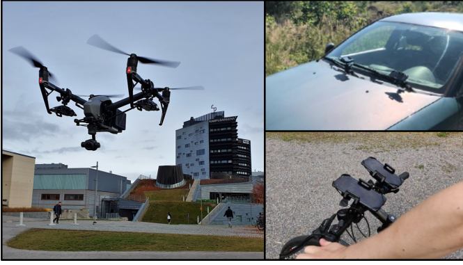
Fig. 2. Different measurement setups: two smart phones attached to a drone, a bicycle, and a car.
