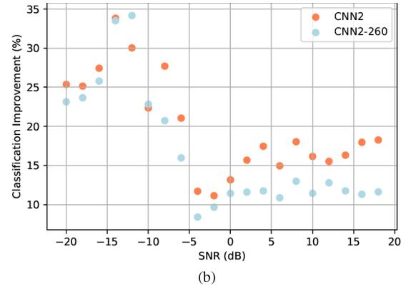
Fig. 2. (a) Classification accuracy and (b) classification improvement (%) of the Complex architecture compared to the CNN2 and CNN2-260 architectures, computed by  $100 \times \frac{Accuracy_{Complex} - Accuracy_{model}}{Accuracy_{model}}$ , as a function of SNR.
