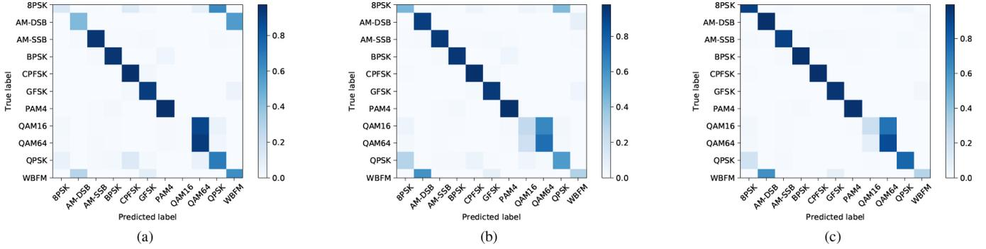
Fig. 5. Confusion matrices at 20 dB for the (a) CNN2, (b) CNN2-260, and (c) Complex architectures. The respective classification accuracies are 68.99%, 73.09%, and 81.58%. In the Complex confusion matrix, the off diagonal noise is greatly reduced. Thus, the features learned through the use of complex convolutions are able to better differentiate the modulations in the presence of high signal strength compared to the other CNN approaches used.
