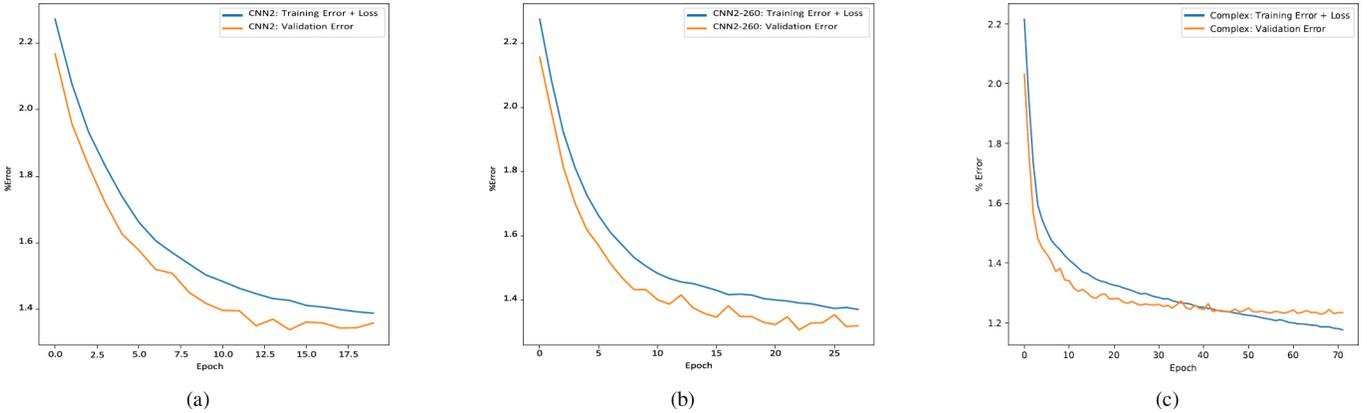
Fig. 6. The training and validation loss curves for the (a) CNN2, (b) CNN2-260, and (c) Complex architectures.
