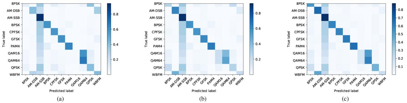
Fig. 3. Average, average across all SNR's, confusion matrices for the (a) CNN2, (b) CNN2-260, and (c) Complex architectures. The respective classification accuracies are 48.45%, 49.63%, and 53.79%.
