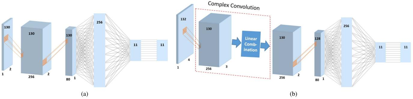
Fig. 1. (a) Schematic of the CNN architecture, CNN2 used to classify modulated I/Q signals in [14]. Please see Table I for the architecture details. (b) Schematic of the Complex architecture, which is CNN2 with modification to compute complex convolutions. For architecture details, see the Table II.
