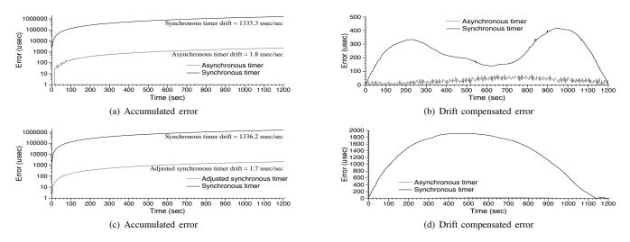
Figure 3. Error between synchronous and asynchronous physical (top) and logical (bottom) timers, without and with drift compensation.
