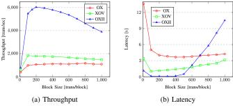
Fig. 5. Throughput/Latency Measurement by Increasing the Block Size
