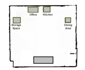
Fig. 3: A slam map of the roamable areas in the indoor environment. Locations of different contexts have been labeled in the map.
