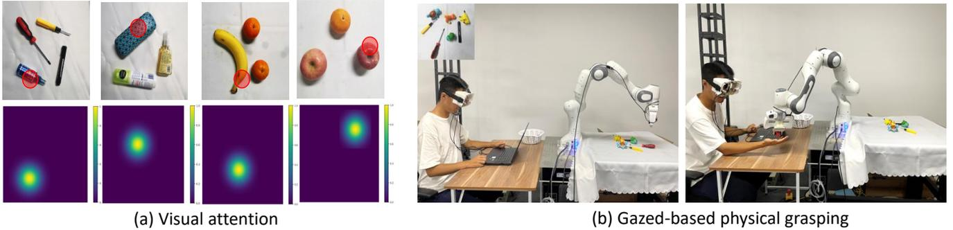
Fig. 4. (a) Visualization of the scene images and the human attention heatmaps captured by our proposed method. From left to right, the human gaze points are the blue bottle, eyeglass box, banana, and apple, respectively. (b) Experiment for real-time gaze-based grasping.
